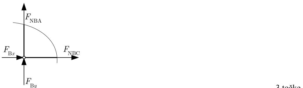
$$\sum F_{ix} = 0 \Rightarrow F_{Bx} + F_{NBC} = 0 \quad \dots \quad 1 \text{ točka}$$
